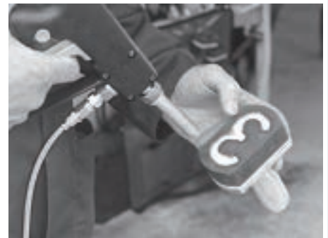
The Brandabull dry ice gun is used to fill the brand digit cavity with dry ice, ready for branding.
