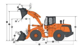
1) Measured to the tip of the bucket teeth or bolt-on edge.
