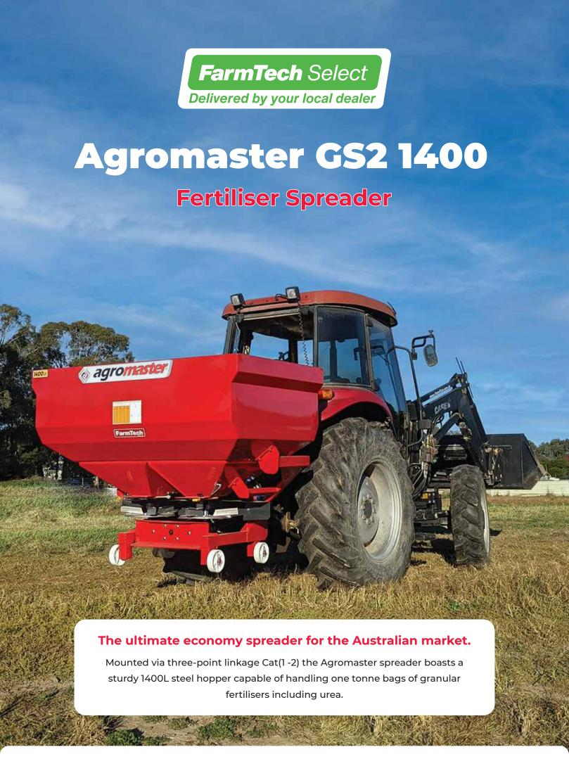
The working width of spread is 18-20 metres via two large stainless-steel discs which are driven by a heavy duty, PTO gearbox (540 RPM).
