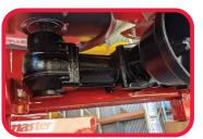
Heavy duty gearbox system powered by tractors PTO shaft
