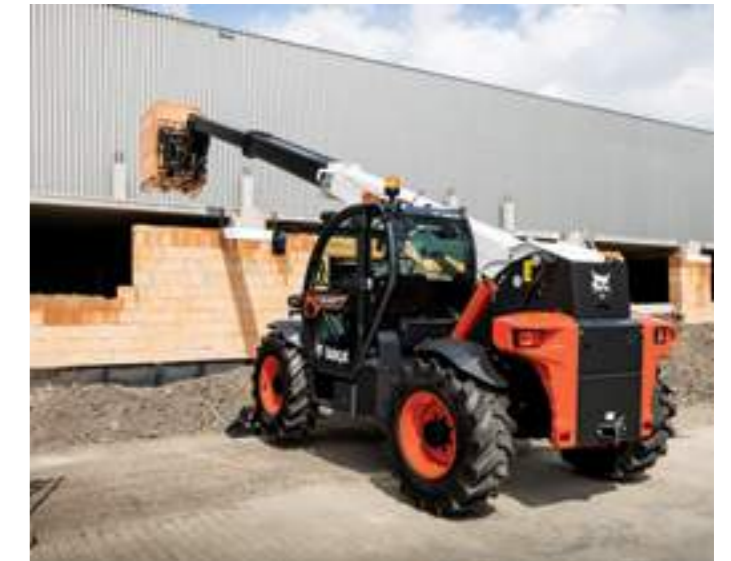
Hydrostatic transmission with dynamic mode for more agility comes as standard for all models.
