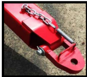
SIMPLE CHAIN AND SPRING ASSEMBLY ON HITCH ALLOWING FOR EASY HOOKUP
