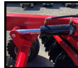
LARGE SINGLE LIFT RAM ON MAIN FRAME
