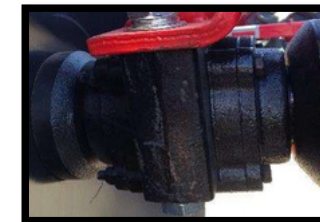
GREASE FILLED BEARING WITH NIPPLE EXTENSION FOR EASY MAINTENANCE
