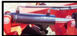
LARGE SINGLE RAM FOR FRAME LIFT
