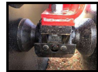
OIL BATH BEARING WITH DUO-CONE SEALS FOR EASY MAINTENANCE
