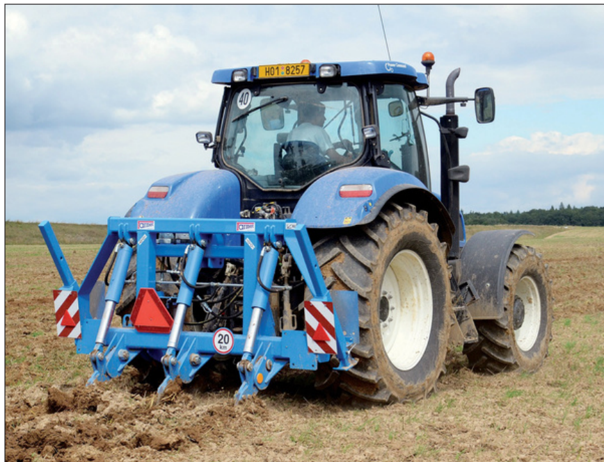
1. Ploughshares in one row for deep cultivation up to the depth of 60 cm.
