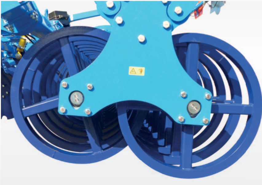
large double rollers \varnothing 680 mm (DVR, DRR)
