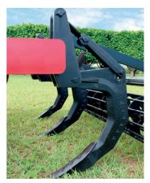
This system is spring loaded on each shank, when a rock, root or stump is hit, the shank will flip back and return to working position when the implement is raised. It does not require any cares for maintenance or adjustments due to its reduced dependence of the moving parts.
