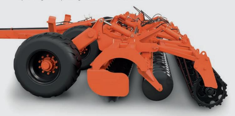
The front disk section cuts, sizes the residue and fractures, lifts and passes the soil and residue mixture to the back disk section, incorporating and leveling the soil profile. The back disk section recuts, resizes and finishes the inversion of the soil and put the mixture back over the soil. The cage roller levels and texturizes the soil.
