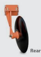
**Rubber torsion suspension system:** the four rubber elements function as damping and provides a pretension, allowing the disc to follow the contour of the land while passing over an obstruction, such as rock. Each shank is independent, allowing for ideal flow of residue.
