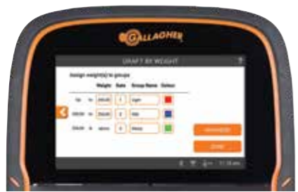
Draft by weight, weight gain or eid list (and traits on the TWR-5 & TW-3)
